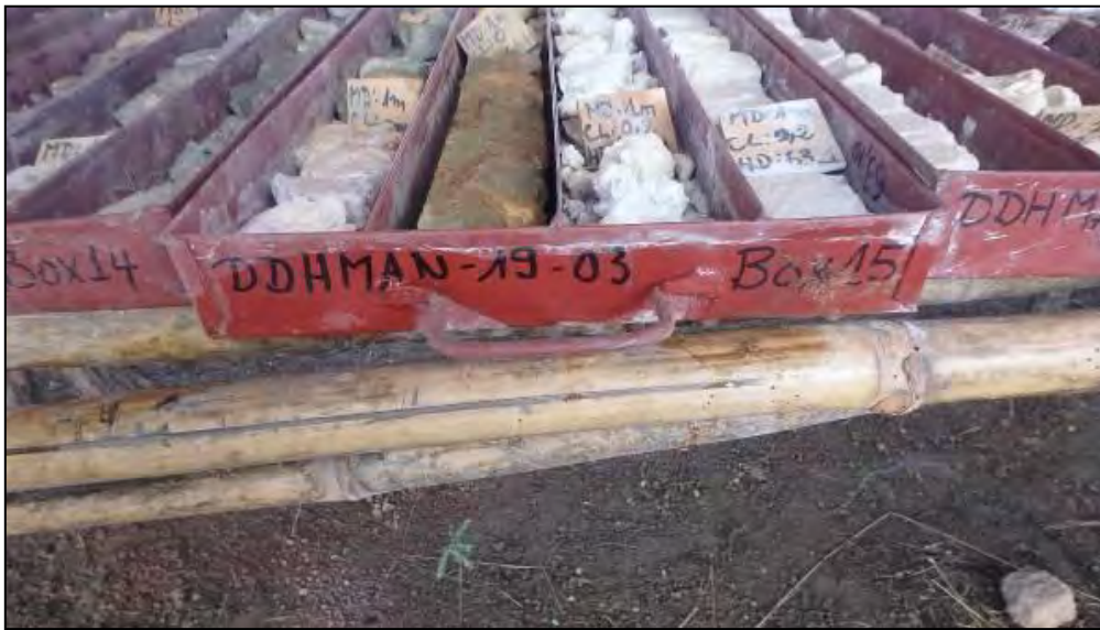
Figure 83. DDHMan-19-03: Dark breccia zone to 61.1 m depth followed by pale bleached saprolite or kaolinite clays
