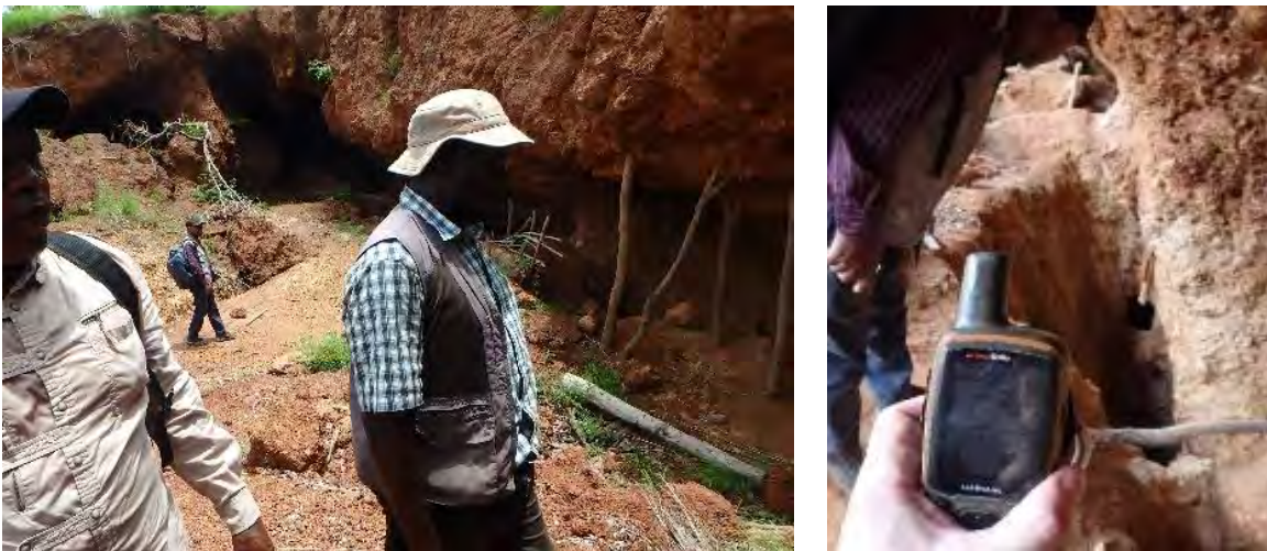
Figure 30. Near-surface exploitation of soft saprolite beneath the laterite cover (left) and deeper workings of steep primary structures to around 20 m (right) – both at Kouroukaida
