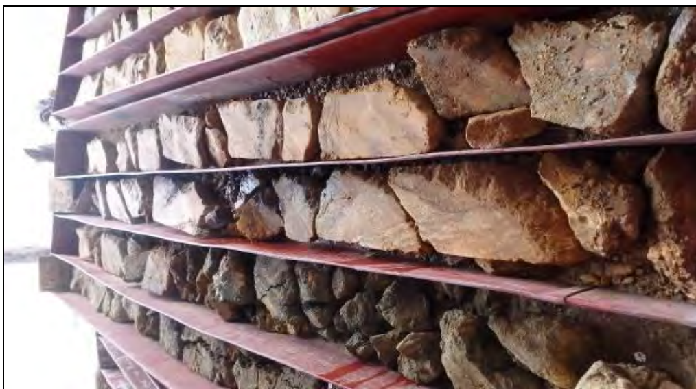
Figure 84. DDHMan-19-04: Quartz veinlets from 80.1 m preceded by darker, more friable, breccia material (lower part of photo)
