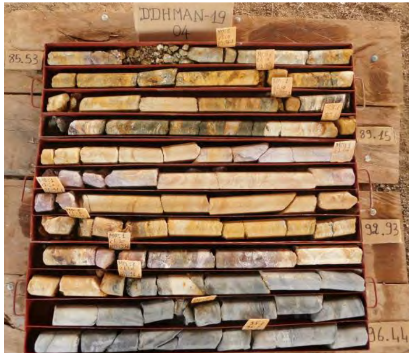
Figure 53. Photo Showing the End of the Mineralised Zone in DDMAN-19-04
