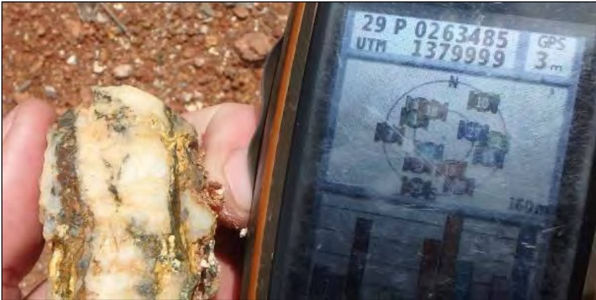
Figure 24. Oxidised sulphides on shale partings along the selvages of thin quartz veins
