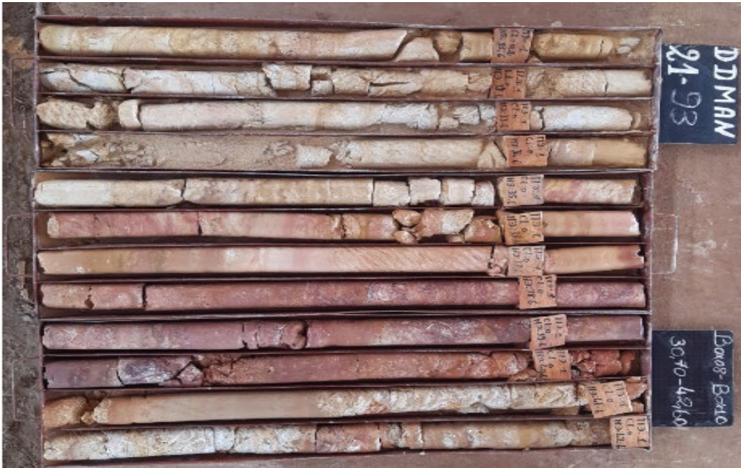
Figure 5: Drill Core Photo DDMAN21-93 showing high grade sections mineralization at MS2
