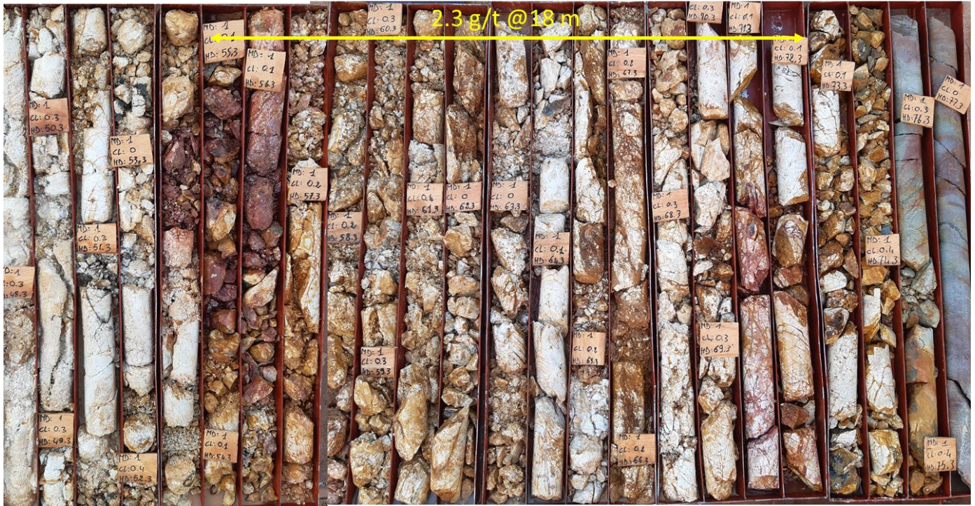
Figure 6: Drill Core Photo DDMan21-106 showing broadly high-grade Sections in saprolite-saprock at MS3.
