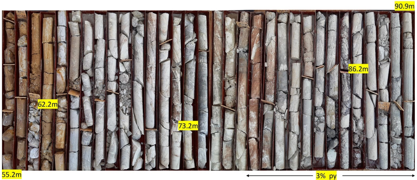
Figure 4: Drill Core Photo DDMan-20-29 showing high grade sections from 55.2-62.2m (gossanous oxidized zone) and 73.2-86.2m (disseminated pyrite zone)
