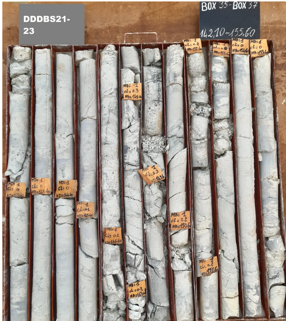
Figure 5: Hole DDDDBS21-023 at Kabaya: Gold Mineralization showing 1.8gpt over 7m
